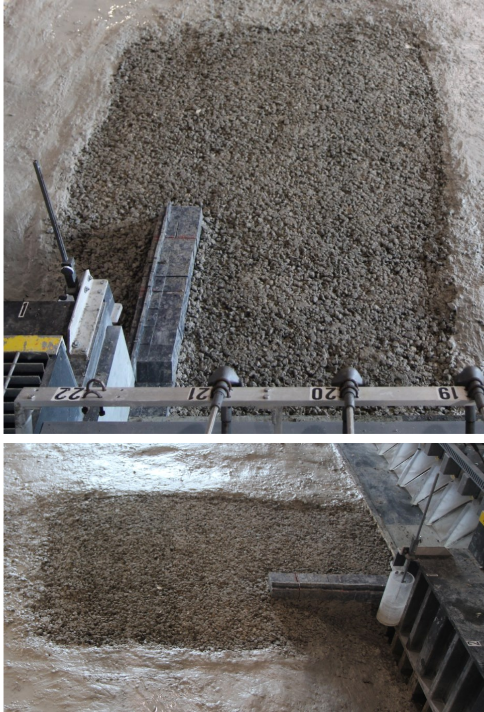
Figure 3-8. Photographs of the initial bathymetry and segmented training wall for the spillbay 22 full open gate scour test
