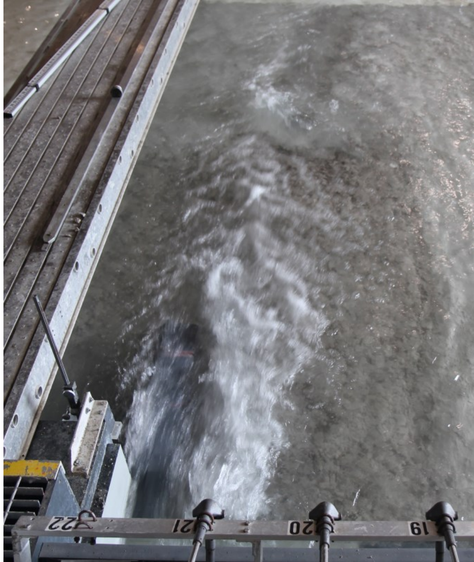
Figure 3-9. Full open gate 22 scour test underway
