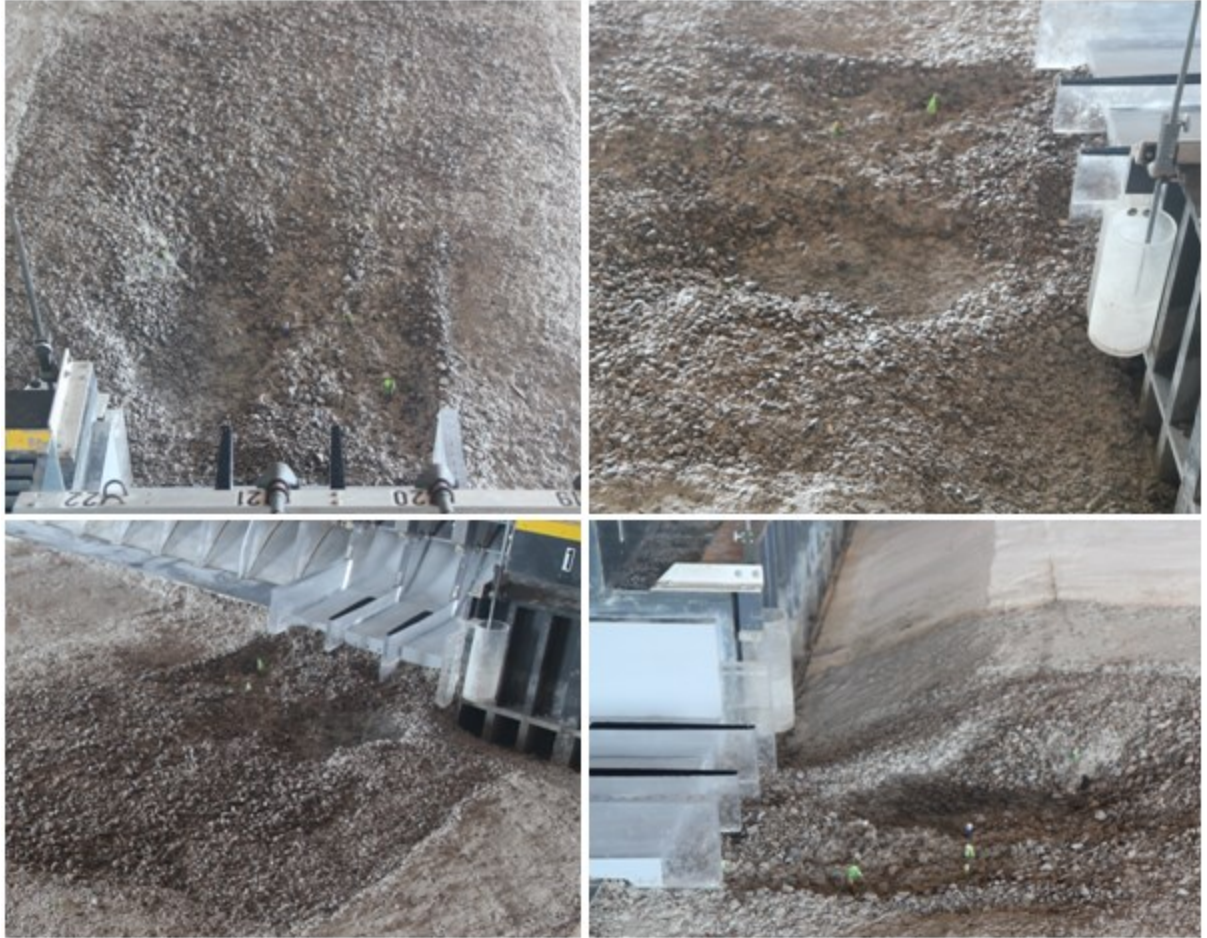
Figure 3-18. Photographs of the final scoured bathymetry for the PRFB scour test
