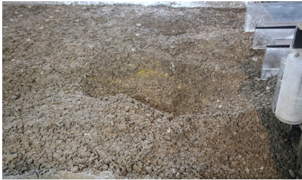
Figure 3-15. Photographs of the initial bathymetry for the PRFB scour test
