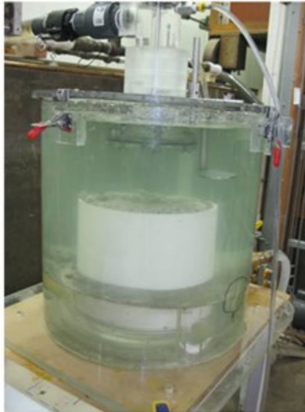
Figure 3-36. JET test underway
