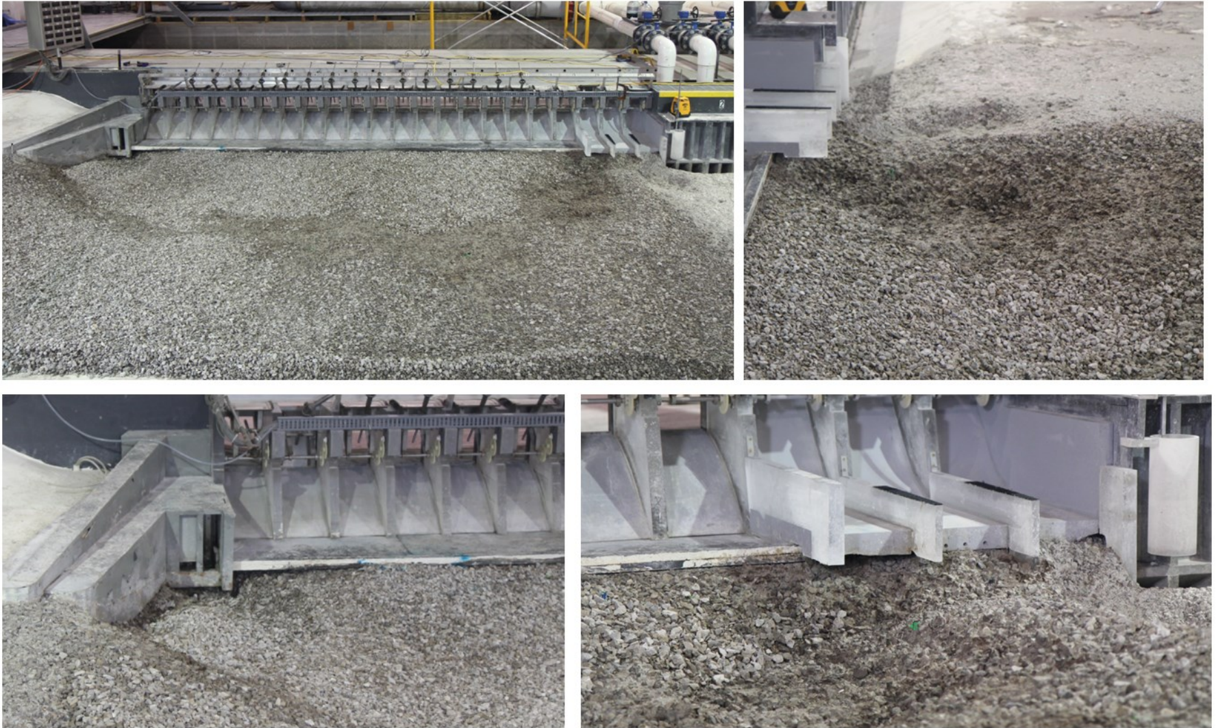
Figure 3-27. Photographs of final scoured bed from PMF scour test
