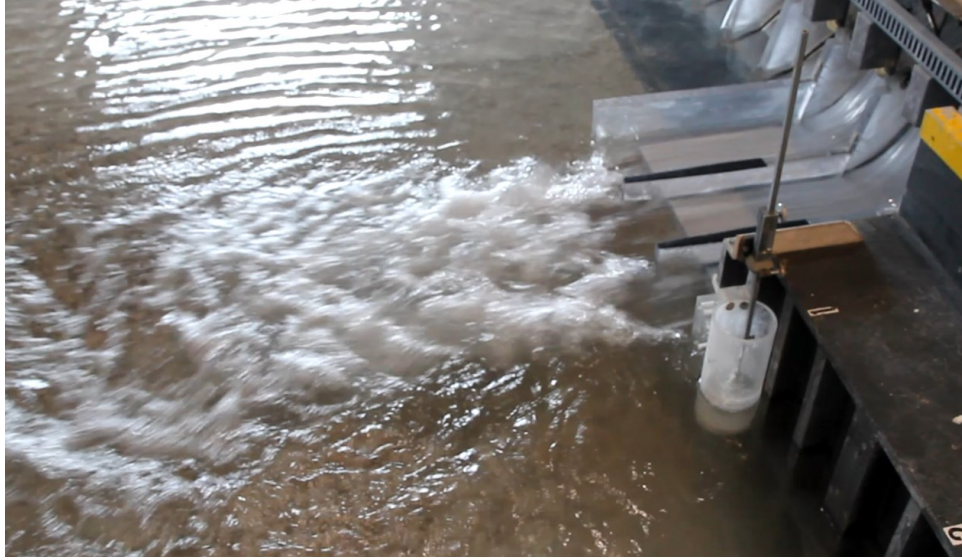
Figure 3-16. PRFB scour test underway
