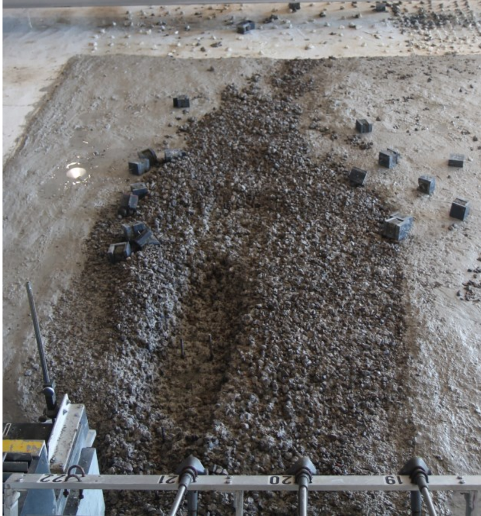
Figure 3-10. Resultant scour hole and final positions of training wall segments
