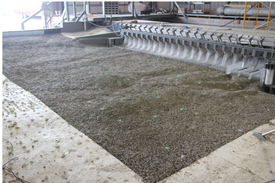
Figure 3-20. Photographs of completed initial bathymetry for PMF scour test
