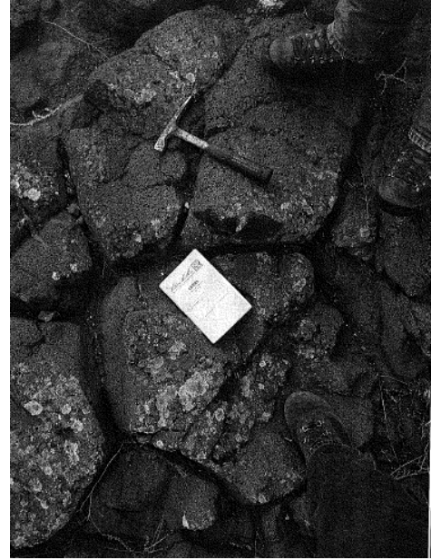
Figure 3-2. Left: View of the top of the columns of the Priest Rapids Member (PR-IV) on the right bank downstream of the Priest Rapids Dam; Right: Priest Rapids Member (PR-IV)-Columns with vesicles (GeoEngineers, Inc., 2005)
